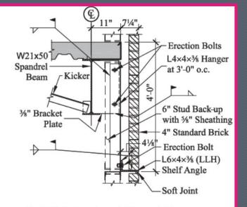
Fig. 7-17. Section of spandrel beam with hanger system.
