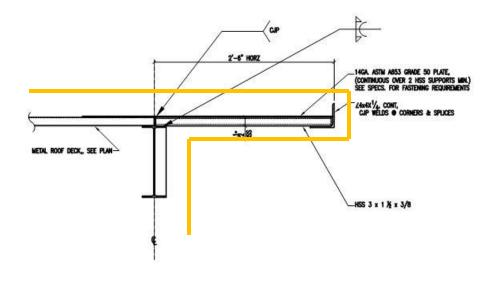
Insulation for portion of framing on inside
