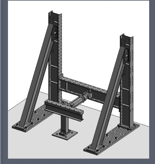
Cantilever test with dead weight as axial loads for roof posts
