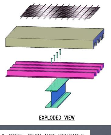
STEEL MESH, CONCRETE, & STEEL DECK NOT REUSABLE
