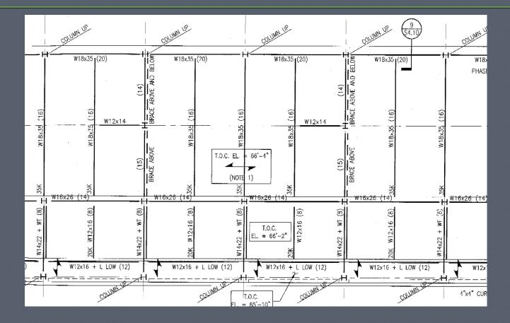
This framing system has repeating bays with similar geometry, beam sizes, and connection types.
