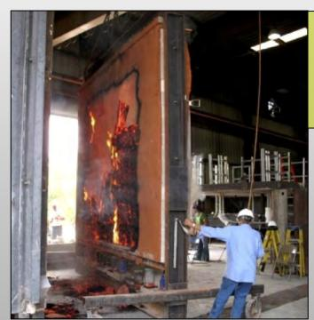
ASTM 2 Hour Fire Rating for Plastered Straw Bale Wall
